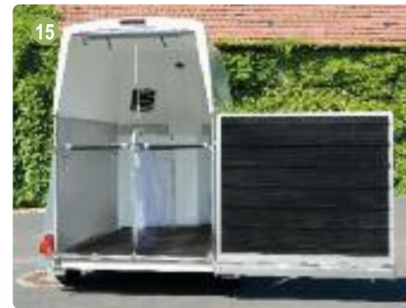
13. Anti-wear mat (not glued to the floor, in front part of trailer, thickness: 18 mm)
